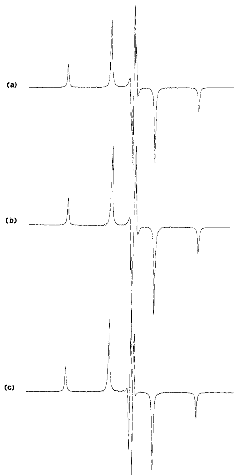
Figure 4. Computer simulated C signals assuming the g and ^{63}\text{Cu} hfc tensors given in the text: (a) Q = 0.00 , g_n = 0.00 ; (b) Q = 2.00 G, g_n = 0.00 ; (c) Q = 0.00 , g_n = 1.48 .
